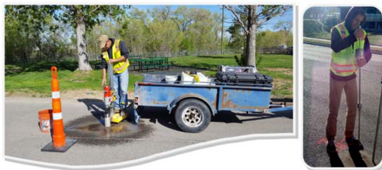
Figure 1. Field Investigation Practices - Coring and Dynamic Cone Penetrometer
